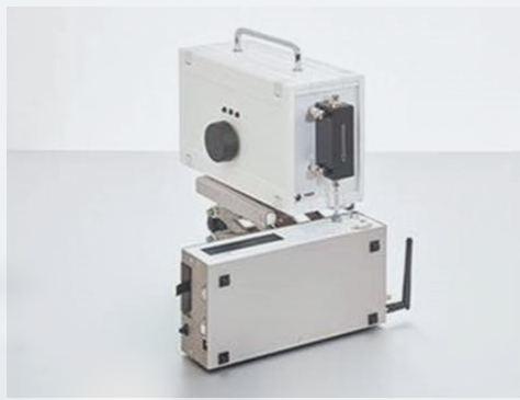
Aerosol spectrometer including dilution unit
